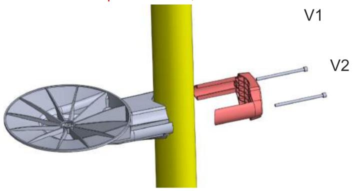
Squiz the support plate to the pillar with the screw V1 and V2
